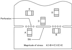
1-3. When breaking PC boards along their perforations, the amount of mechanical stress on the inductors can vary according to the method used. The following methods are listed in order from least stressful to most stressful: push-back, slit, V-grooving, and perforation. Thus, any ideal SMD inductor layout must also consider the PCB splitting procedure.
